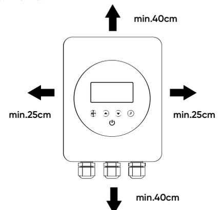
Mark the hole locations on the wall, drill and insert the expansion plugs supplied, fit the screws and hang the device on the screws.
